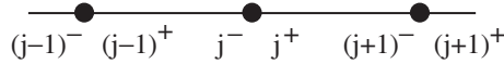
Figure 2. Node j corresponds to the coincident node pair (j^-/j^+) , j = 2, 3, \dots, m .
